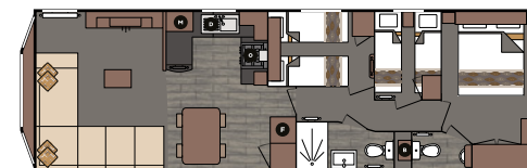
38 X 12 3B Bed Sizes: King size 1905mm x 1525mm, 2 x Single 1830mm x 685mm & 2 x Single 1830mm x 610mm
